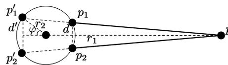
Figure 4. For the spike at  $p$  we consider the affine hulls of the edges adjacent to  $p$ . The intersection of these affine hulls with  $C_2$  define  $p'_1$  and  $p'_2$ . The point  $q$  can lie in any of the spikes spanned by the segment  $p'_1 p'_2$ .
