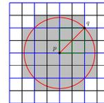
Figure 2: A point  $p$  is selected as a representative for a quadtree cell, denoted by the smaller bold green square of width  $w_i$ . In the worst case, the furthest representative,  $q$ , of the parent square of  $p$ , denoted by the larger bold green square, is a distance  $2\sqrt{2}w_i$  from  $p$ . Consequently,  $p$ ’s transmission range interferes with at most 32 cells of the quadtree at its level.
