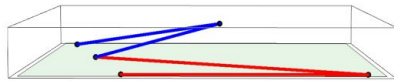
Figure 5: The maxspan configuration with links L_3 and L_4 rotated out of \Pi_1 . The maxspan is |v_0v_2| + |v_2v_4| .
